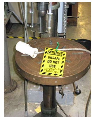
Faulty Drill Press tagged out
